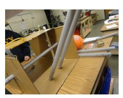
The two uptakes are a row of 1/8" polycord that rolls basketballs against a pair of dead rails. The second uptake's dead rails telescope to facilitate the shooter's variable angle.
